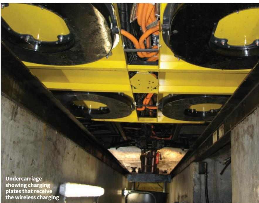
Undercarriage showing charging plates that receive the wireless charging
